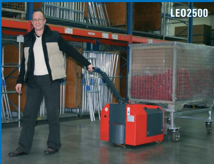
LEO2500 for safe handling, acceleration, and braking of payloads up to 2500 kg
